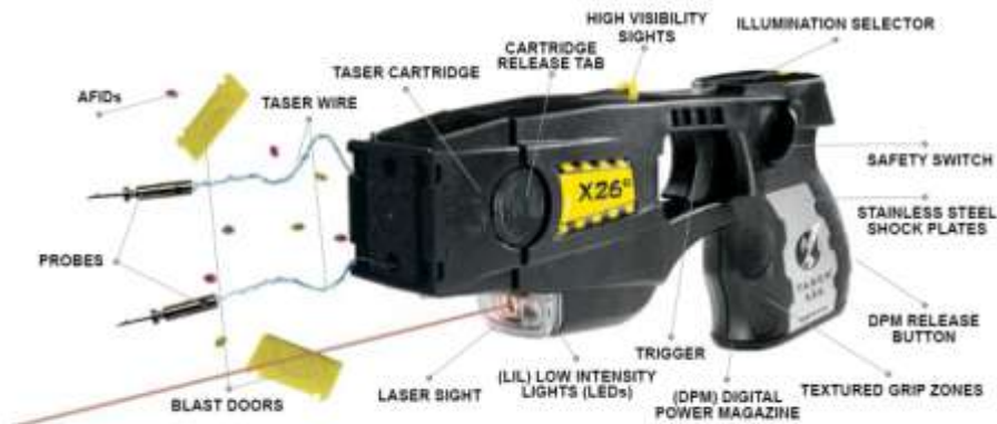
Figure 1: Taser International's X26 electromuscular incapacitation device
